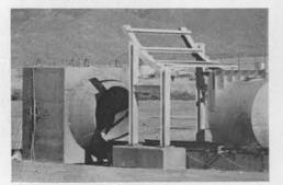
TANK, on front of sled, approaches target at nearly 100 mph.
